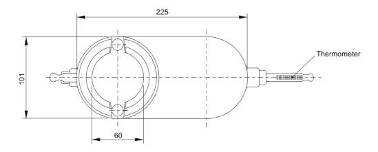
Figure 6 – Standard Williams type penetrometer
